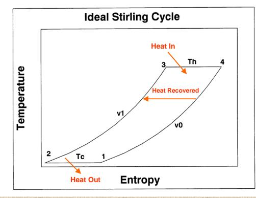
1-2 Constant Temperature Compression from v0 to v1with Heat Removal 2-3 Constant Volume Heat Addition (Regenerator) 3-4 Constant Temperature Expansion from v1 to v0 with Heat Addition 4-1 Constant Volume Heat Removal (Regenerator) Heat In =  $Q_{in} = T_h \Delta S$ Heat Out =  $Q_{out} = T_c \Delta S$ Work =  $Q_{in} - Q_{out} = (T_h - T_c) \Delta S$ Efficiency =  $\eta$  = Work/Heat In =  $(T_h - T_c) \Delta S/Th \Delta S$
